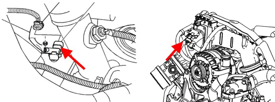
**Figure 1 - '02-'04 (Left) and 04.5-09 (Right) MAP Sensor Locations**
